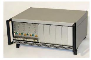
Applications for the LTBiS are laser diode burn-in and laser diode life test. The LTBiS consists of two hardware
